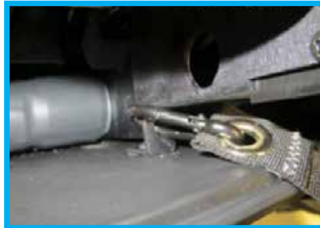
Figure 12. Attach Tether to Retract Bracket
