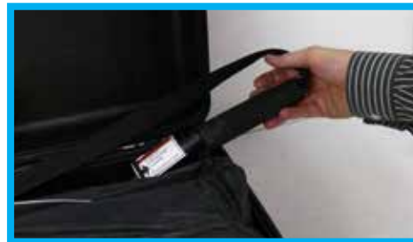
Figure 23. Insert Drogue in Launch Tube
