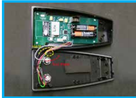
Figure 28. Reposition Front and Back Pieces of the Case
