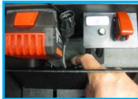
Figure 24. Locate Reset Button Facing the Power Switch
